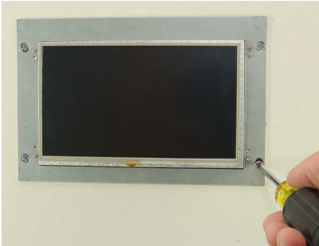
Figure 13 Touch Screen Assembly Installation
