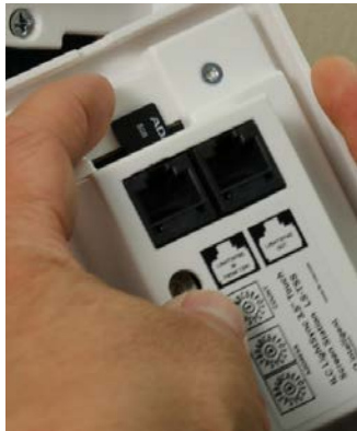
Figure 17 SD Card Installation
