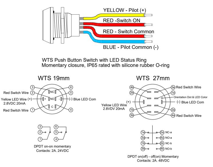
The Wet Location Touch Switch hardwire assembly will come with 1, 2 or 3 push buttons in a single gang stainless steel faceplate with Neoprene gasket. Weatherproof wirenuts provided for extending the wire from wet location installation to the control inputs installed in a dry location.
