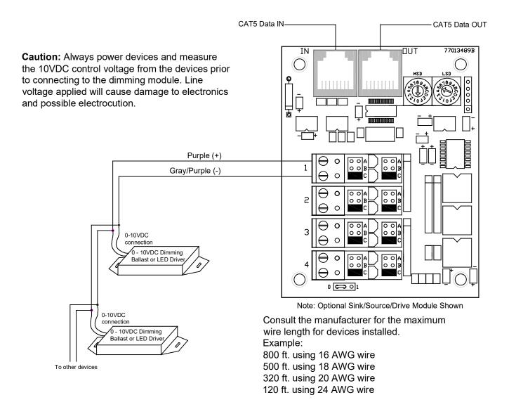
The LightSync Isolated Dimming Module provides 4 independent zones for controlling ballasts, LED drivers or other devices that have 0 - 10VDC control. Each control port can control up to 200 ballasts parallel connected based on a typical current of .5mA each, with a maximum of 100mA per output channel or dimming zone. Consult manufacture for current requirements and recommended wiring practices for class 2 wiring.
