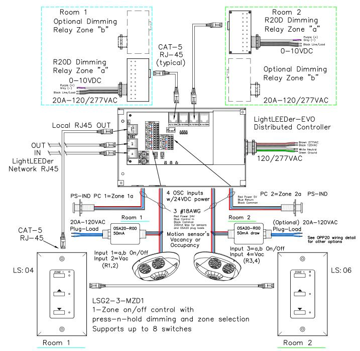
LL—EVO panel used for controlling 2 independent rooms with 1 zones each. LightLEEDer EVO 4—zone panel with 2—remotely mounted R20D relays. Two daylight sensor inputs w/independent zone settings, motion sensor inputs For up to 4 independent zones, or hardwire switch. Optional plug—load relay, Local LightSync output for Multi—Zone Dimmer (MZD) station with raise/lower press—n—hold dimming, supports 1 to 8 LightSync input devices.
