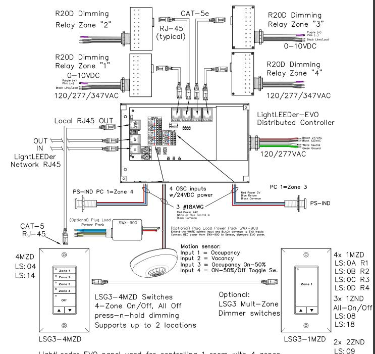
LightLeeder EVO panel used for controlling 1 room with 4 zones. Remotely mounted R20D relays, for Open Office spaces.
