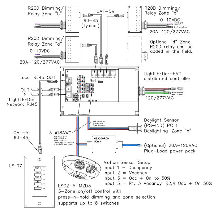
LightLEEDer EVO 3—Zone panel with 3—remotly mounted R20D relays. Daylight sensor with independent zone settings, Motion sensor inputs for up to 4 independent zones or local hardwire switch. Optional plug—load relay. Local LightSync output for Multi—Zone Dimmer (MZD) station with raise/lower press—n—hold dimming, supports from 1 to 8 LightSync input devices.
