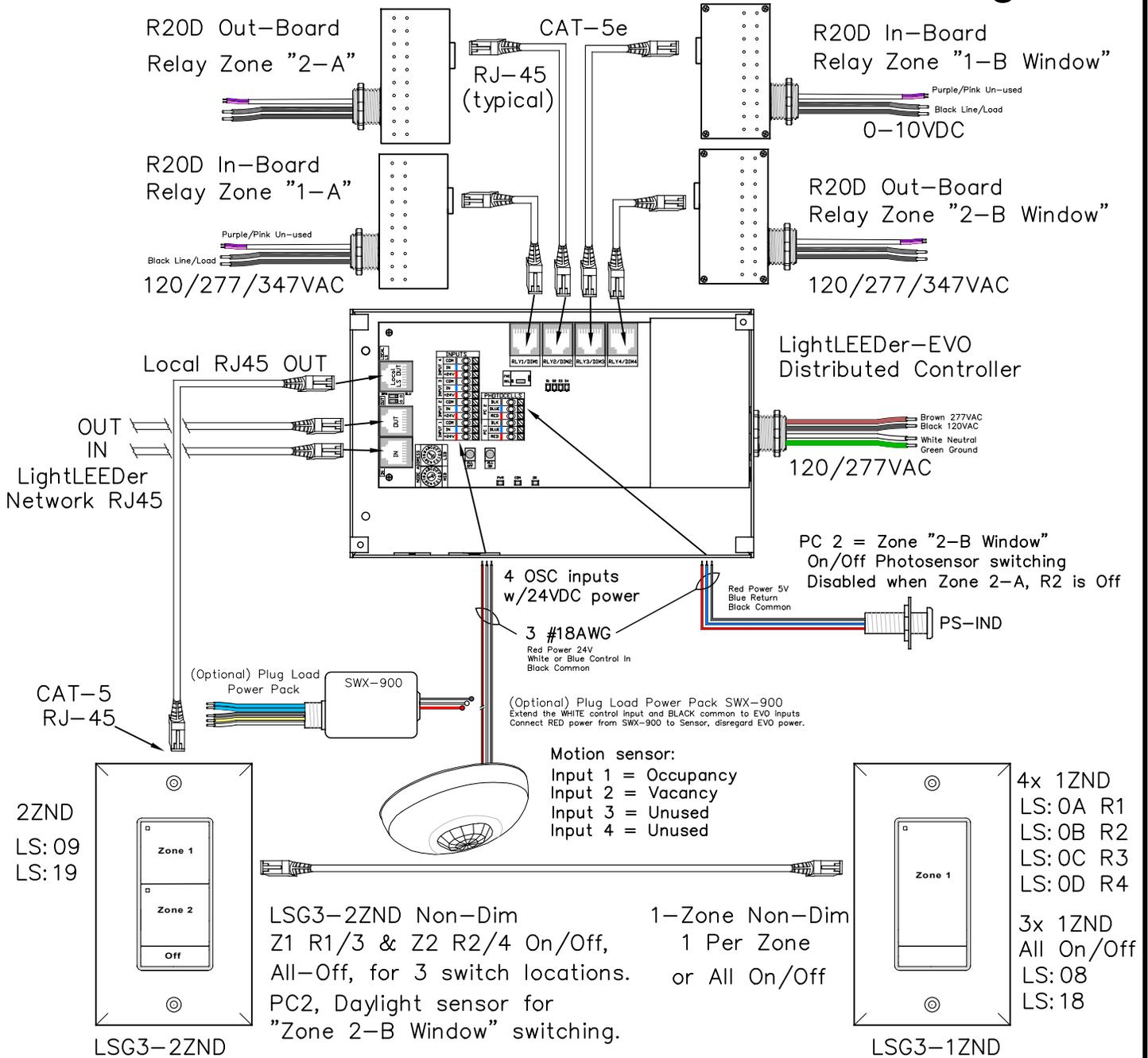
LightLEEDer EVO panel used for controlling 1 room with 2 zones A/B switching
