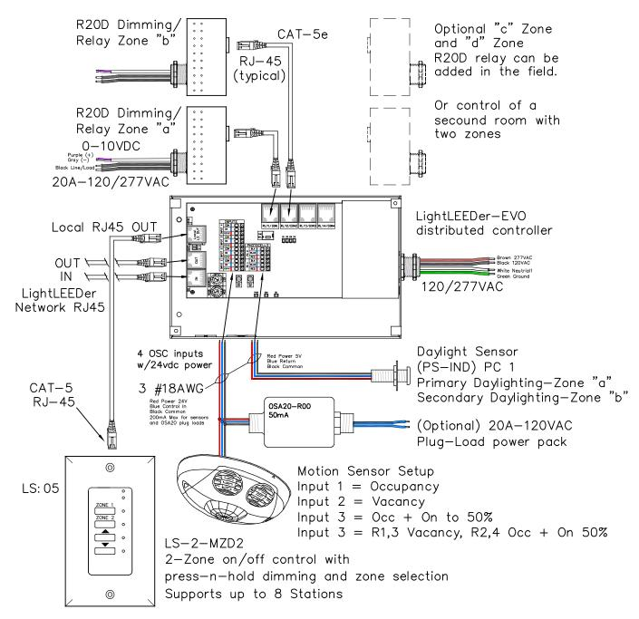
LightLEEDer EVO 2—Zone panel with 2—remotly mounted R20D relays Daylight sensor with independent zone settings, Motion sensor inputs for up to 4 independent zones or local hardwire switch. Optional plug—load relay. Local LightSync output for Multi Zone Dimmer station (MZD) with raise/lower press—n—hold dimming, supports from 1 to 8 LightSync input devices.
