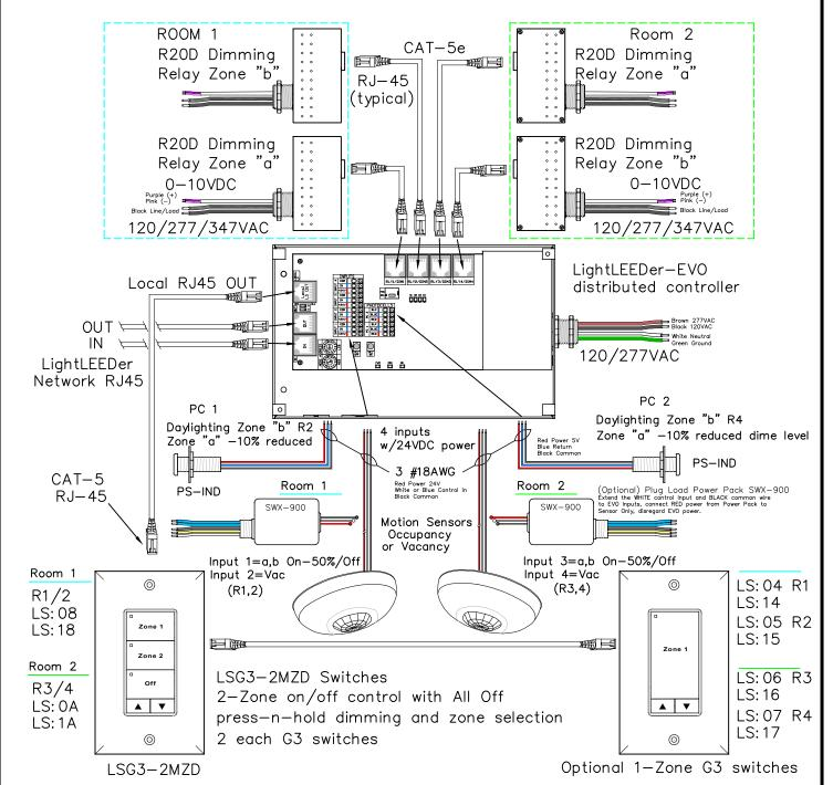
LL-EVO panel used for controlling 2 independent rooms with 2 zones each LightLEEDer EVO 4-Zone panel with 4-remotely mounted R20D relays. Two daylight sensor inputs with independent zone settings, motion sensor inputs two for each room with Occupancy-50% or Vacancy operation. Local LightSync MZD digital Multi-Zone Dimmer station with raise/lower for 1 or 2 Zone with press-n-hold dimming. Supports 1 to 8 LightSync input devices.
