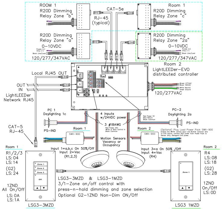
LL-EVO panel used for controlling 2 independent rooms with 3/1 zones LightLEEDer EVO 4-Zone panel with 4-remotely mounted R20D relays. Two daylight sensor inputs with independent zone settings, motion sensor inputs for up to 4 independent zones, or hardwire switch. Optional plug-load relay, Local LightSync output for Multi-Zone Dimmer MZD station with raise/lower press-n-hold dimming. Supports 1 to 8 LightSync input devices.
