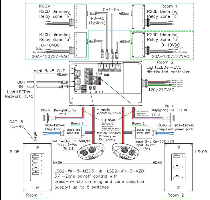
LL-EVO panel used for controlling 2 independent rooms with 2 zones each LightLEEDer EVO 4-Zone panel with 4-remotely mounted R20D relays. Two daylight sensor inputs with independent zone settings, motion sensor inputs for up to 4 independent zones, or hardwire switch. Optional plug-load relay, Local LightSync output for Multi-Zone Dimmer station (MZD) with raise/lower press-n-hold dimming, supports 1 to 8 LightSync input devices.
