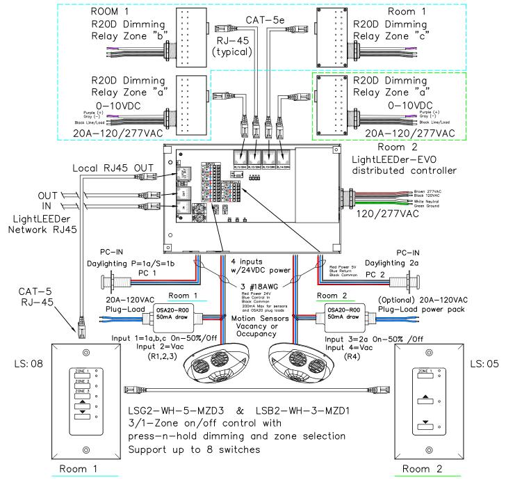
LL—EVO panel used for controlling 2 independent rooms with 2 zones each LightLEEDer EVO 4—Zone panel with 4—remotely mounted R20D relays. Two daylight sensor inputs w/independent zone settings, motion sensor inputs for up to 4 independent zones, or hardwire switch. Optional plug—load relay, Local LightSync output for Multi—Zone Dimmer station (MZD) with raise/lower press—n—hold dimming, supports 1 to 8 LightSync input devices.
