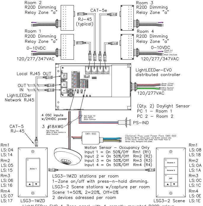
LightLEEDer EVO 4—Zone panel with 4—remotly mounted R20D relays, On-board Daylight Sensor inputs for Rm 1&2 (Remote input LS:11&12 for RM3&4). Occupancy On at 50% /Off 1-4 for Rm 1-4, Local LightSync port for LSG3 or G2 Multi-Zone Dimmer station MZD with raise/lower or 2-Scene stations press—n—hold dimming. Supports from 1 to 8 LightSync input devices.
