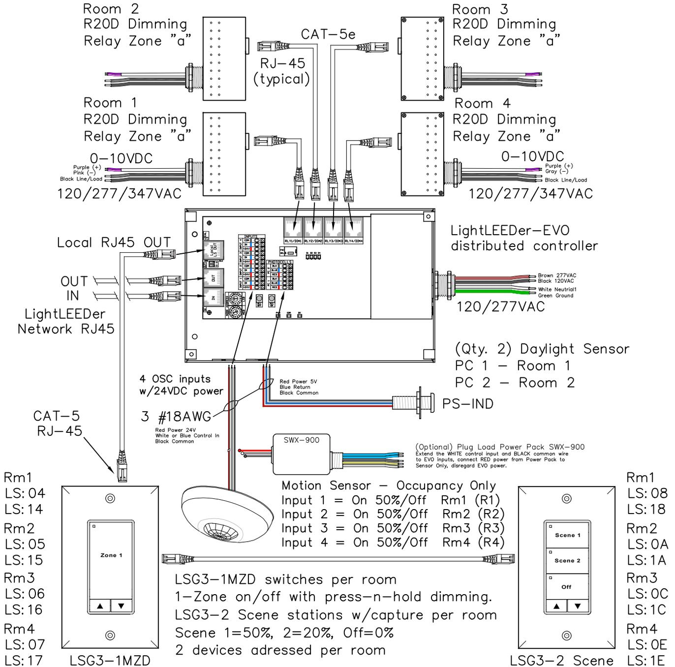
LightLEEDer EVO 4-Zone panel with 4-remotely mounted R20D relays, On-board Daylight Sensor inputs for Rm 1&2 (Remote input LS:11&12 for RM3&4). Occupancy On at 50% /Off 1-4 for Rm 1-4 , Local LightSync port for LSG3 Multi-Zone Dimmer switches with raise/lower or 2-Scene switches press-n-hold dimming. Supports from 1 to 8 LightSync input devices. Optional LSIM modules for hardwire On/Off switch 3-wire (LS:13) 2-Wire (LS:23)
