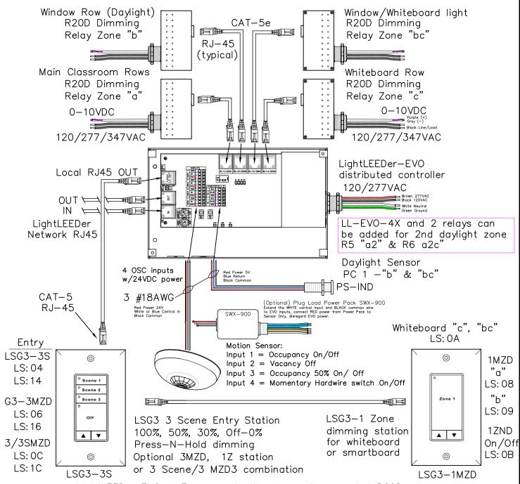
LightLEEDer EVO 4—Zone panel with 4—remotly mounted R20D relays Daylight sensor for window row lighting control, motion sensor inputs for Occupancy On/Off, Vacancy Off, Occ 50% On/Off or local hardwire switch. Local LightSync devices for Scene or MZD stations with raise/lower dimming All On/Off, and Whiteboard control. Supports up 8 LightSync input devices.
