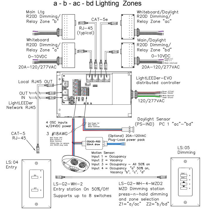
LightLEEDer EVO 4—Zone panel with 4—remotly mounted R20D relays Daylight Sensor with independent zone settings, Motion sensor inputs for up to 4 independent zones or local hardwire switch. Optional plug—load relay. Local LightSync output for Multi—Zone Dimmer station (MZD) with raise/lower press—n—hold dimming, supports from 1 to 8 LightSync input devices.
