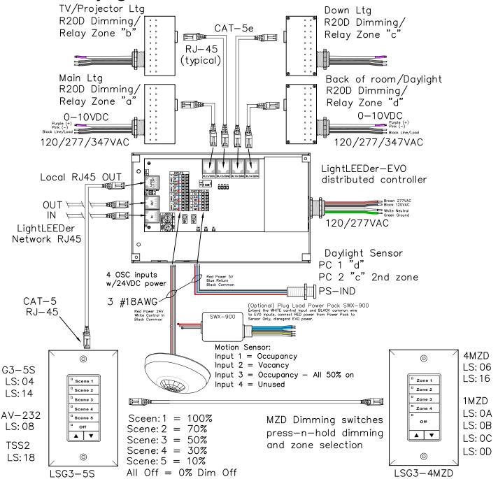
LightLEEDer EVO 4—Zone panel with 4—remotly mounted R20D relays, Daylight Sensor w/ Independent zone settings, Motion sensor inputs for Occupancy, Vacancy or Occupancy on at 50%. Optional plug—load relay. Local LightSync G3 Scene switches w/Capture or Multi—Zone Dimmer switches with raise/lower press—n—hold dimming, optional singe zone switches, TS2 Touch Screen and AV interface. Supports from 1 to 8 LightSync devices.
