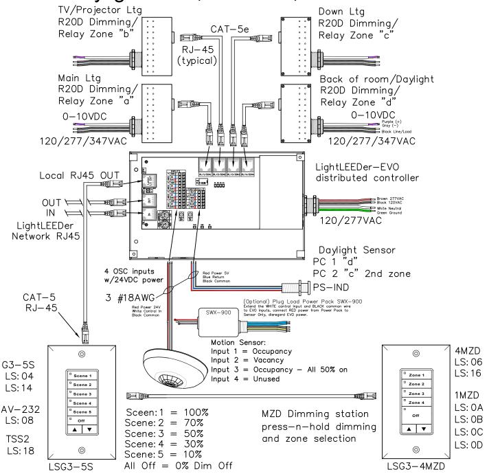
LightLEEDer EVO 4—Zone panel with 4—remotly mounted R20D relays, Daylight Sensor w/ Independent zone settings, Motion sensor inputs for Occupancy, Vacancy or Occupancy on at 50%. Optional plug—load relay. Local LightSync G3 Scene stations w/Capture or Multi—Zone Dimmer station with raise/lower press—n—hold dimming, optional singe zone stations, TSS2 Touch Screen and AV interface. Supports from 1 to 8 LightSync devices.
