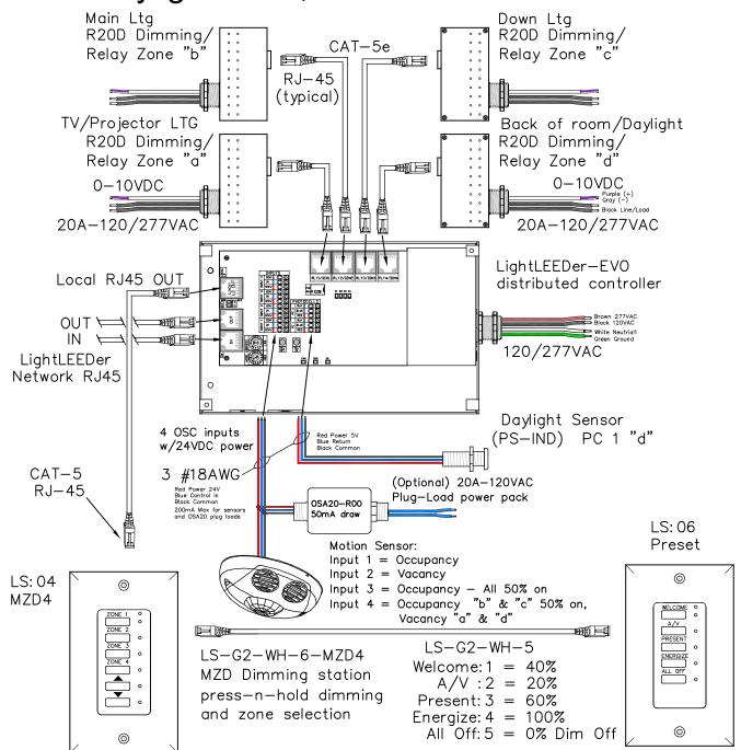
LightLEEDer EVO 4—Zone panel with 4—remotly mounted R20D relays Daylight Sensor w/ Independent zone settings, Motion sensor inputs for up to 4 independent zones or local hardwire switch. Optional plug—load relay. Local LightSync output for Multi—Zone Dimmer station (MZD) with raise/lower press—n—hold dimming, supports from 1 to 8 LightSync input devices.
