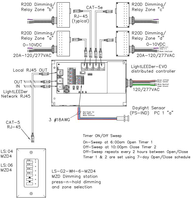
LightLEEDer EVO 4—Zone panel with 4—remotly mounted R20D relays Daylight Sensor w/ Independent zone settings, Motion sensor inputs for up to 4 independent zones or local hardwire switch. Optional plug—load relay. Local LightSync output for Multi—Zone Dimmer station (MZD) with raise/lower press—n—hold dimming, supports from 1 to 8 LightSync input devices.
