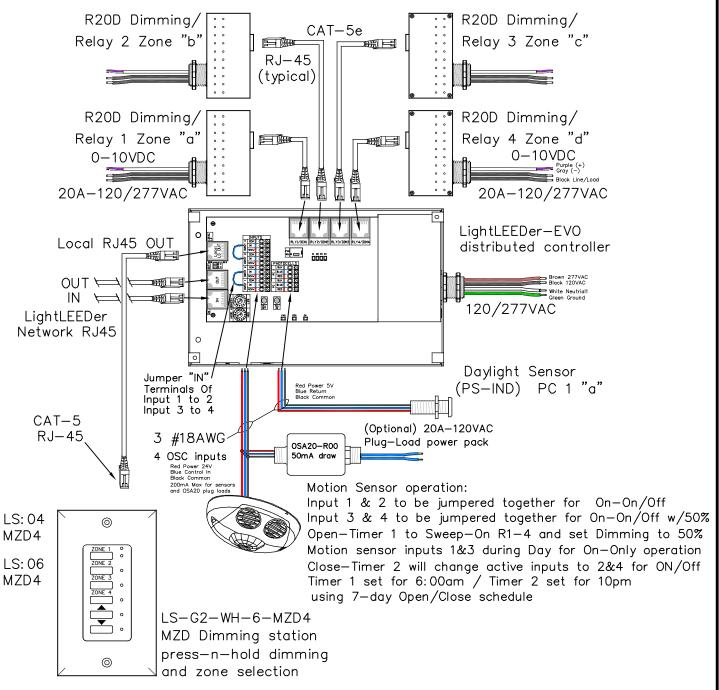
LightLEEDer EVO 4—Zone panel with 4—remotly mounted R20D relays Daylight Sensor w/ Independent zone settings, Motion sensor inputs for up to 4 independent zones or local hardwire switch. Optional Plug—load relay. Local LightSync output for Multi—Zone Dimmer station with Raise/Lower press—n—hold dimming, supports from 1 to 8 LightSync input devices.
