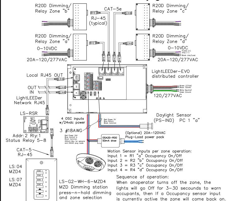
LightLEEDer EVO 4—zone panel with 4—remotly mounted R20D relays Daylight Sensor w/ Independent zone settings, Motion sensor inputs for up to 4 independent zones or local hardwire switch. Optional Plug—load relay. Local LightSync output for Multi—Zone Dimmer (MZD) station with raise/lower press—n—hold dimming, supports from 1 to 8 LightSync input devices.
