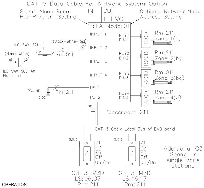
Switch On/Off with dimming
