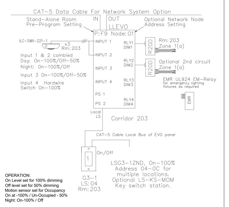
Photocell can be added to limits max level in daylight zones using relay output 2, If Windows or Skylights are present . Pre-Program F9
