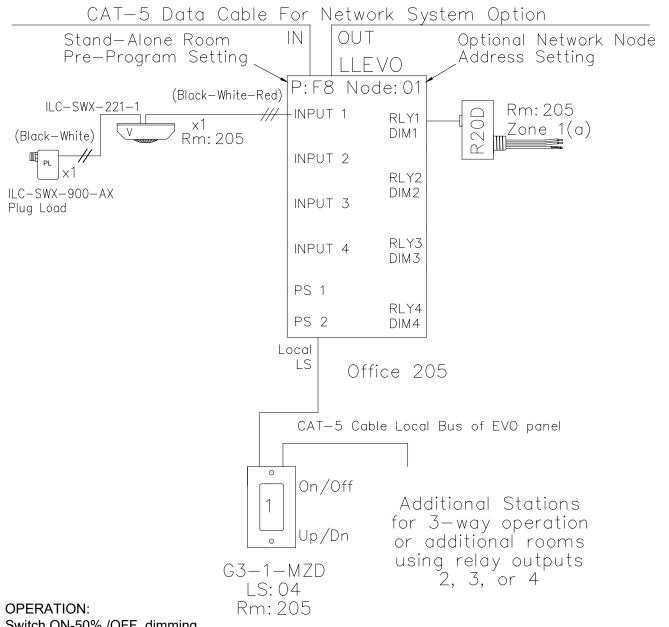
Switch ON-50% /OFF, dimming Motion sensor set for Vacancy Plug-load relay for 120V outlets operated by motion sensor on/off. Pre-Program F8
