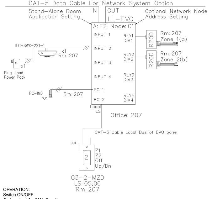
On Level set for 50% dimming Motion sensor set for Vacancy Photocell limits max level in daylight zones Plug-load relay for 120V outlets operated by motion sensor on/off.
