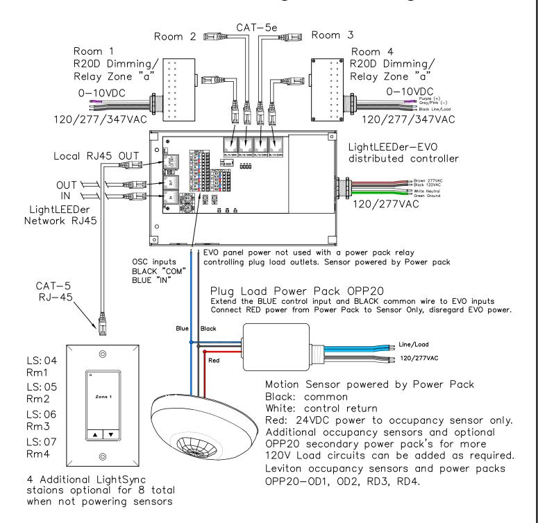
LightLEEDer EVO 4—Zone panel with 4—remotly mounted R20D relays See EVO Lighting Application F7 and F8 for Switch and R20D relay details
