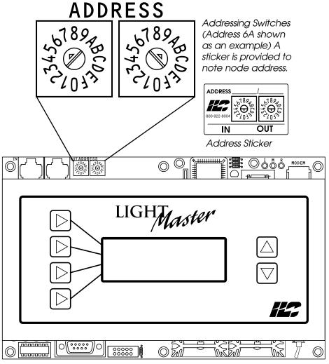
LightMaster Processor Board and Keypad
