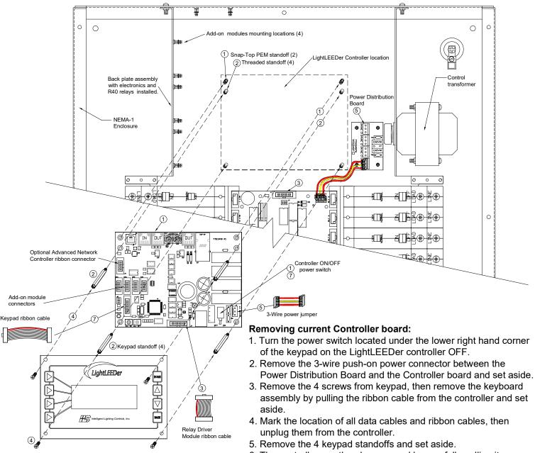
6. The controller can then be removed by carefully pulling it straight off from the back plane Snap-Top PEMs holding the board.
