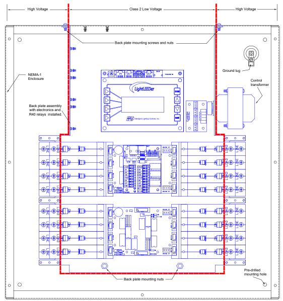
Note: Electronic components must be protected from falling debris during installation. This can be done by using a cardboard shield to cover the electronics, or the interior back plate and electronics can be removed and stored in the shipping box until the enclosure and electrical conduit is installed.
