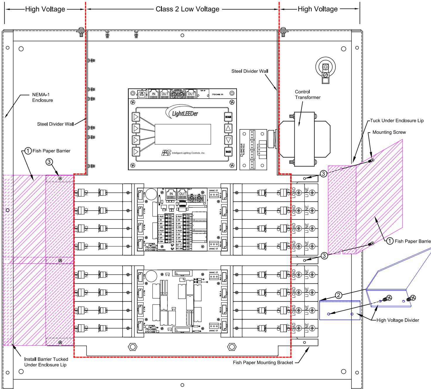
The right and left sides of the enclosure can be dedicated to different line voltages (120 or 277V) and would not require a high voltage divider. If the left or right relay section needs to be separated from top to bottom a high voltage divider can be field installed.
