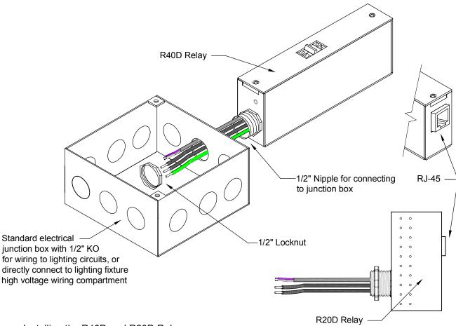
Installing the R40D and R20D Relay:
