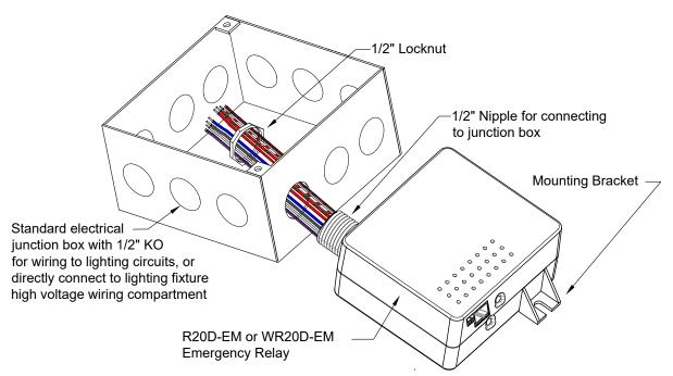
Installing the R20D-EM or WR20D-EM Relay:
