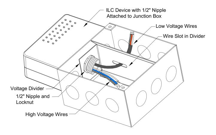
This junction box divider may be required for separation of line volt circuits, normal from emergency circuits, or Class-2 control wiring from line voltage Class-1 wiring to meet NEC Code requirements.
