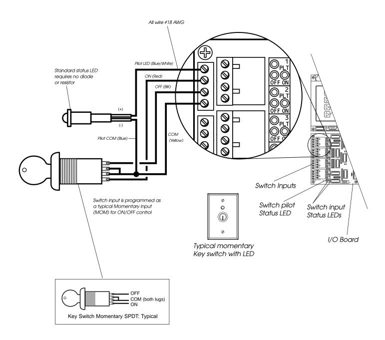
Typical Momentary 3-wire ON/OFF Key Switch Wiring
