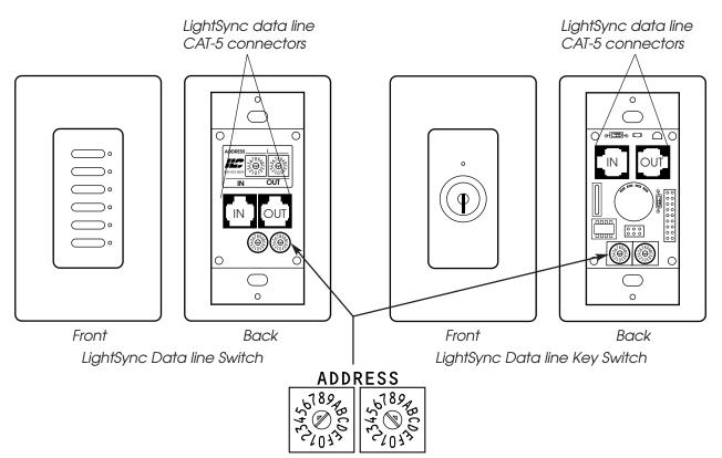
Addressing Switches (Address 6A shown as an example) A sticker is provided to note node address.
