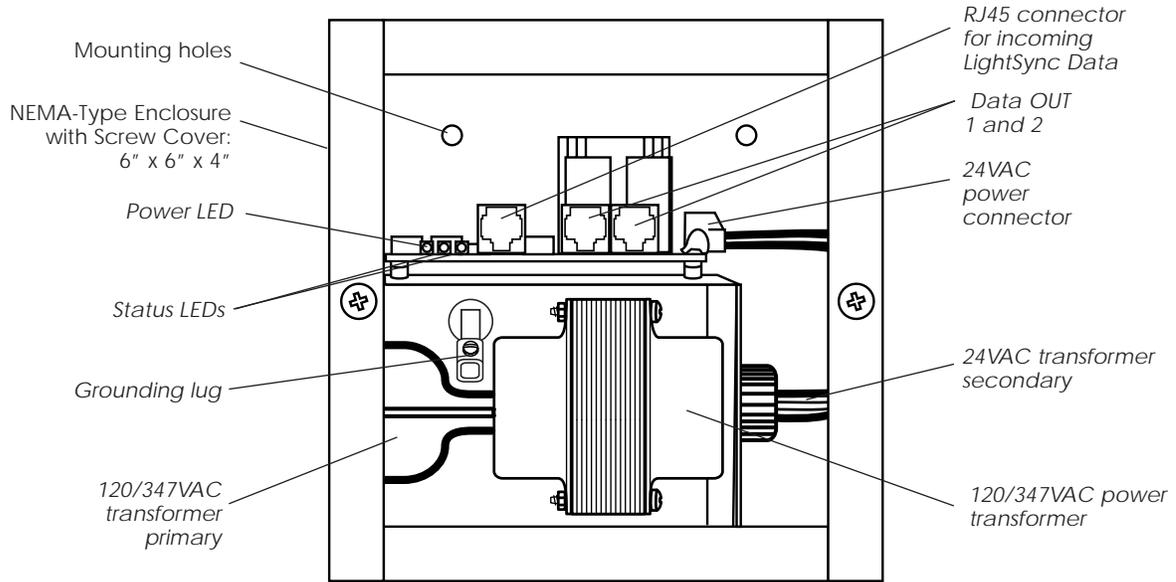
LightSync Power Supply Repeater (PSR) Detail
