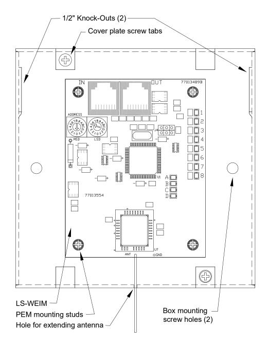
Install LS-WEIM using the provided 4-11/16" junction box. Connect to ILC LightLEEDer network using CAT-5 data cable. Mount device so that antenna protrudes downward unobstructed. Keep clear from other 902MHz equipment, preferred location would be where the antenna extends down into open air below the ceiling tile,allowing a 100' radius for EnOcean switch stations and occupancy sensors devices.
