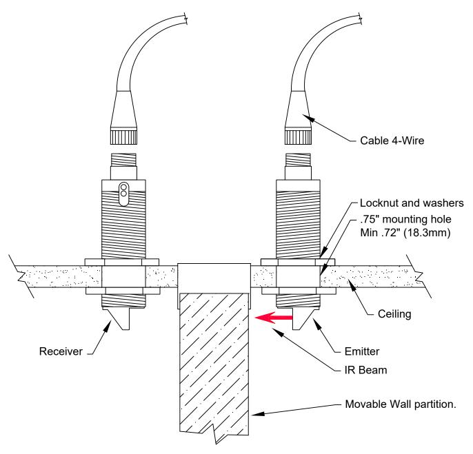
Install Photoelectric partition sensors in ceiling on both sides of movable wall partition by drilling a .75" hole and securing sensors with the locknut and washers provided.
