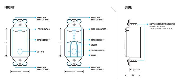
\*\* SENSOR FACE IS FIELD REMOVABLE IN ORDER TO CHANGE COLORS. CONTACT FACTORY FOR ADDITIONAL FACES
