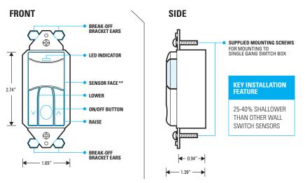
\*\* SENSOR FACE IS FIELD REMOVABLE IN ORDER TO CHANGE COLORS. CONTACT FACTORY FOR ADDITIONAL FACES
