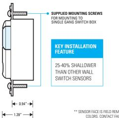
\*\* SENSOR FACE IS FIELD REMOVABLE IN ORDER TO CHANGE COLORS. CONTACT FACTORY FOR ADDITIONAL FACES
