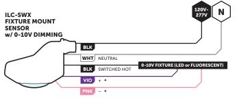
\* VIO/PNK DIMMING WIRES (0-10V) SHOULD BE TREATED AS CLASS 1
