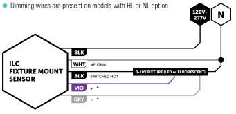
\* VIO/GRY DIMMING WIRES (0-10V) SHOULD BE TREATED AS CLASS 1
