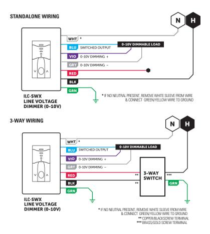
NOTE: This product is UL listed and meets NEC 404.2(c) & 404.22 guidelines regarding powering over ground & current leakage. Powering over ground is permitted for replacement / retrofit onl.
