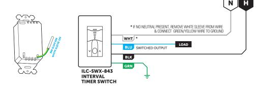
NOTE: This product is UL listed and meets NEC 404.2(c) & 404.22 guidelines regarding powering over ground & current leakage. Powering over ground is permitted for replacement / retrofit only.
