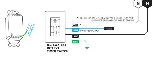
NOTE: This product is UL listed and meets NEC 404.2(c) & 404.22 guidelines regarding powering over ground & current leakage. Powering over ground is permitted for replacement / retrofit only.
