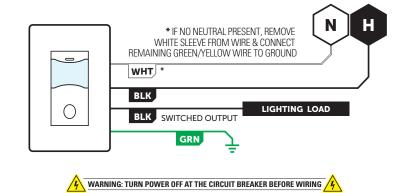
NOTE: This product is UL listed and meets NEC 404.2(c) & 404.22 guidelines regarding powering over ground & current leakage. Powering over ground is permitted for replacement / retrofit only.
