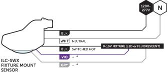
\* VIO/GRY DIMMING WIRES (0-10V) SHOULD BE TREATED AS CLASS 1
